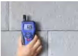
Measure moisture of wall material with non-invasive Pinless technology
